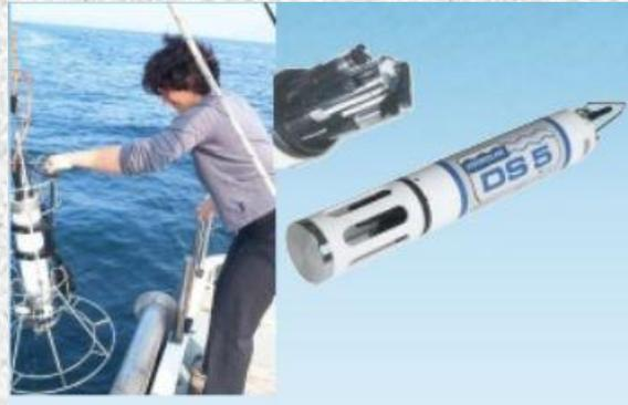
Example of a multiparameter sensor used for the measurement of depth, temperature etc.
